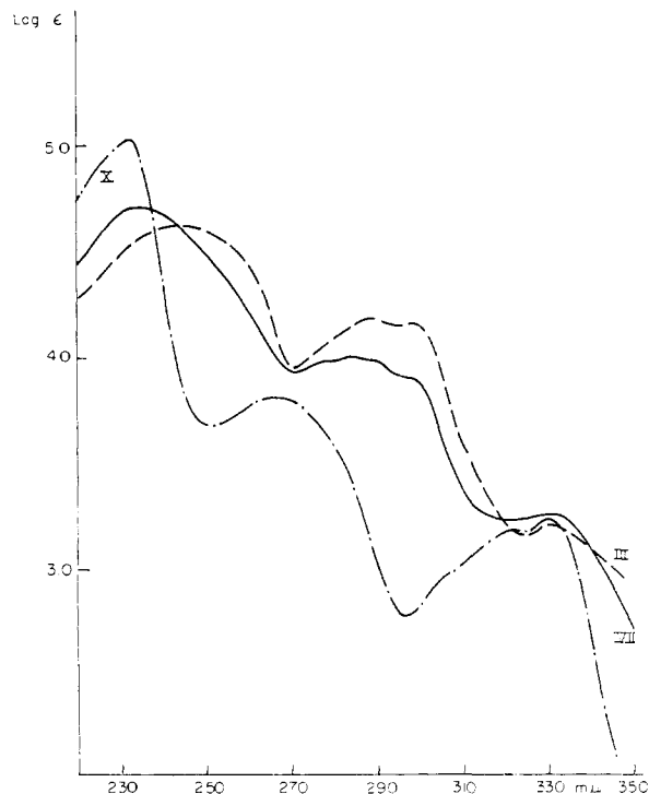
Fig. 1.—Ultraviolet absorption spectra of unsaturated and saturated 2-methoxynaphthyl acids.
